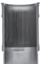
Severely Scuffed Liner
