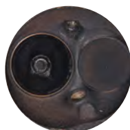
Cylinder head before P.i. treatment.
