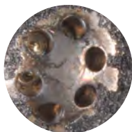
Injector after one P.i. treatment.
