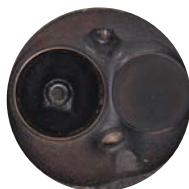
Cylinder head before P.i. treatment.
