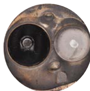
Cylinder head after one P.i. treatment.
